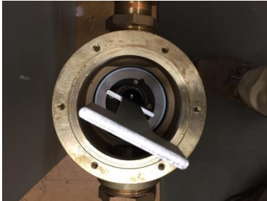
Loosen Sleeve Locking Nut (Use fork side of tool on the upper notches)
