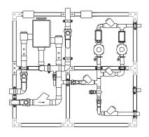
2 PUMPS R Redundant recirculation pump
