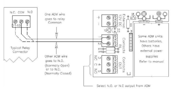
This is the hookup from a relay (contact) output of an LMS-188-4P-BMS, or other device, to the RDU.
