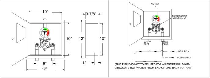
CAUTION! It may be necessary to recirculate the tempered water to the eye/face wash should the piping be exposed to excessive hot or cold conditions. Consult factory for proper piping.
