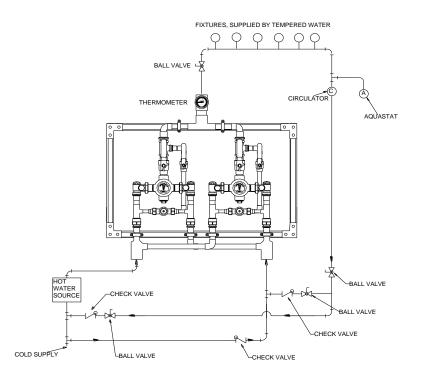
**CAUTION!** All thermostatic water mixing valves have limitations. They will NOT provide the desired accuracy outside of their flow capacity range. Consult the Flow Capacity Chart and DO NOT OVERSIZE. Minimum flow must be no less than as indicated.
