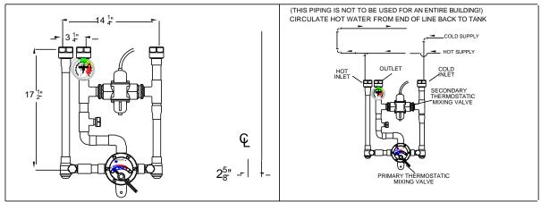
CAUTION! It may be necessary to recirculate the tempered water to the emergency shower should the piping be exposed to excessive hot or cold conditions. Consult factory for proper piping.
