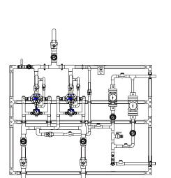
**2 PUMPS R**Redundant recirculation pump
