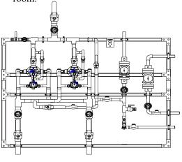
**2 PUMPS H**High temperature loop recirculation pump
