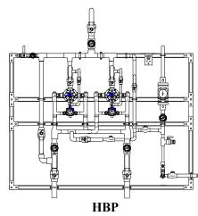
High temperature by-pass flush with locking ball valve
