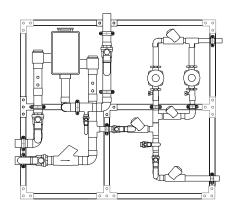
2 PUMPS R Redundant recirculation pump
