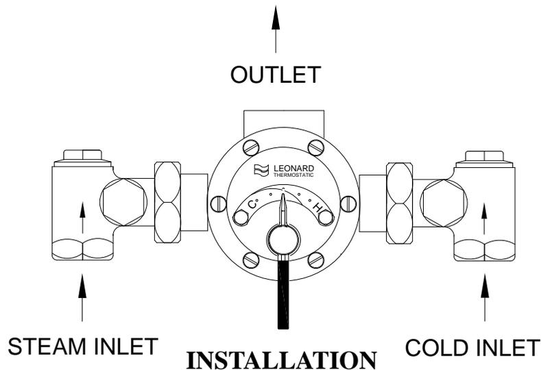
1. Valve should be installed at a location where it can easily be cleaned, adjusted or repaired.
