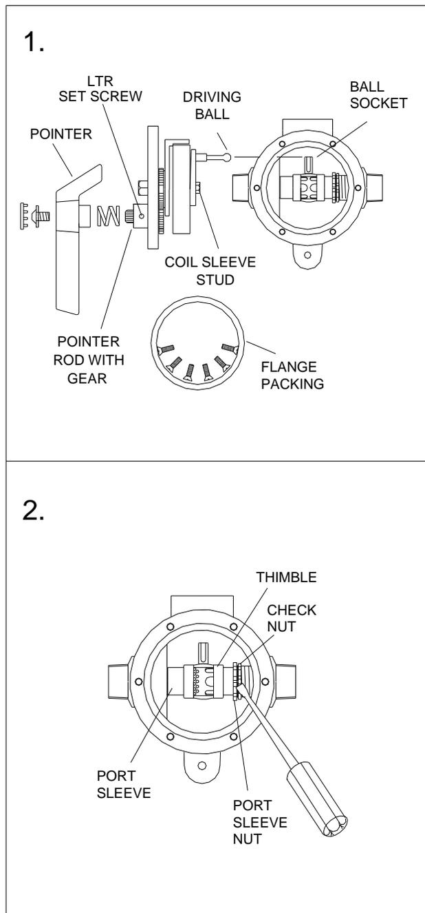
**REMEMBER! THIS IS A CONTROL DEVICE WHICH MUST BE CLEANED AND MAINTAINED ON A REGULAR BASIS. (SEE MAINTENANCE GUIDE AND RECORD, MGR-1000).**
