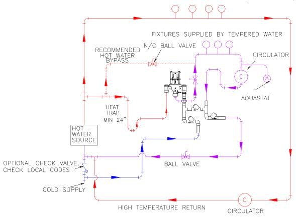
**CAUTION!** All thermostatic water mixing valves have limitations. They will NOT provide the desired accuracy outside of their flow capacity range. Consult the Flow Capacity Chart and DO NOT OVERSIZE. Minimum flow must be no less than as indicated.
