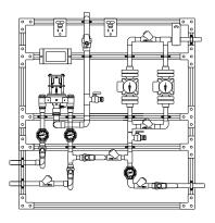
2 PUMPS R Redundant recirculation pump
