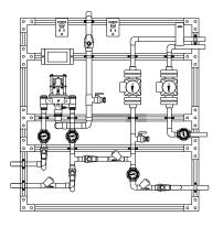
**2 PUMPS H** High temperature loop recirculation pump
