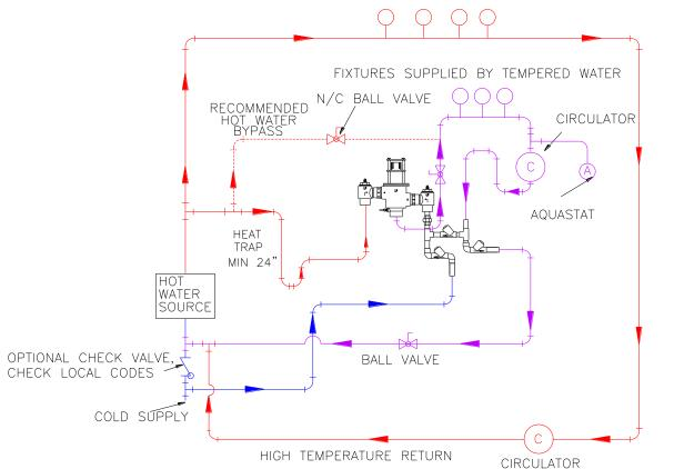
**CAUTION!** All thermostatic water mixing valves have limitations. They will NOT provide the desired accuracy outside of their flow capacity range. Consult the Flow Capacity Chart and DO NOT OVERSIZE. Minimum flow must be no less than as indicated.
