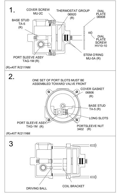
After installation, adjustment, and cleaning, always check the temperature of the valve when turned to full **HOT** per the warning on the front page, using a thermometer. Also check and if necessary adjust the temperature of the hot water source. **EXCESSIVELY HOT WATER (OVER 110°F) IS DANGEROUS AND MAY CAUSE SCALDING!!**
