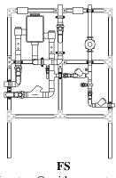
Megatron<sup>®</sup> with separate legs to floor to support the unit without hangers.
