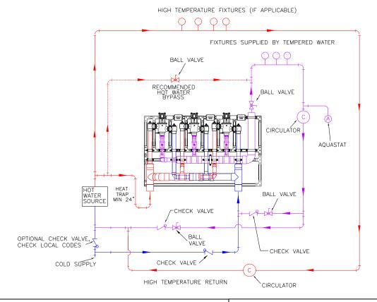
**CAUTION!** All thermostatic water mixing valves have limitations. They will NOT provide the desired accuracy outside of their flow capacity range. Consult the Flow Capacity Chart and DO NOT OVERSIZE. Minimum flow must be no less than as indicated.
