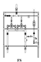
Megatron® with separate legs to the floor (shipped loose), attaches to channel of existing megatron to support the unit without hangers.
