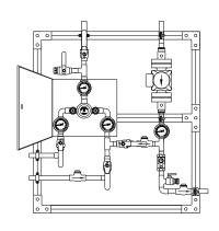
CAB Megatron® with cabinet around mixing valve
