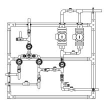
2 PUMPS R Redundant recirculation pump
