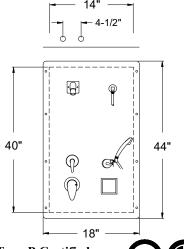
Valve is ASSE 1016 – Type P Certified Valve is CSA B.125-16 – Type P Certified
