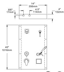
Valve is ASSE 1016 – Type P Certified Valve is CSA B.125-16 – Type P Certified
