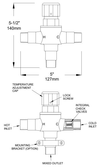
This product is certified to meet Low Lead requirements of wetted surface area containing less than 0.25% lead by weight
