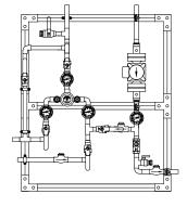
HBP High temperature by-pass flush with locking ball valve
