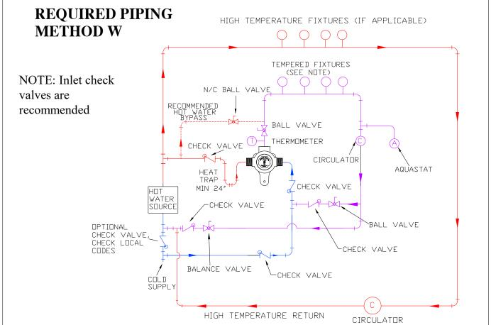
**CAUTION!** All thermostatic water mixing valves have limitations. They will NOT provide the desired accuracy outside of their flow capacity range. Consult the Flow Capacity Chart and DO NOT OVERSIZE. Minimum flow must be no less than as indicated.
