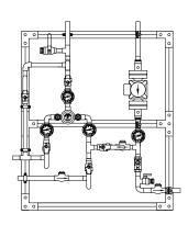
**HBP** High temperature by-pass flush with locking ball valve
