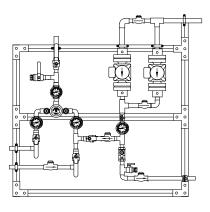
2 PUMPS R Redundant recirculation pump
