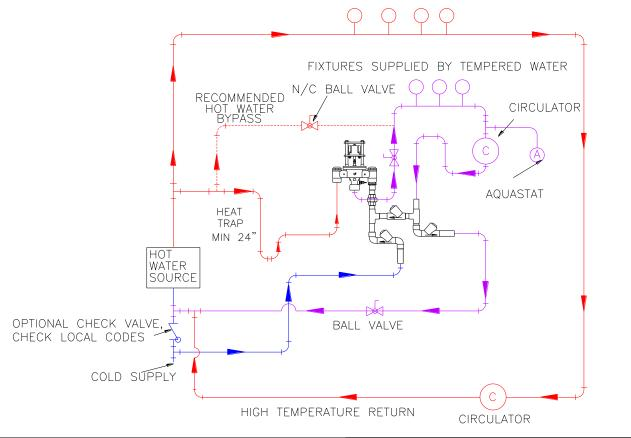
CAUTION! All thermostatic water mixing valves have limitations. They will NOTE: Flow rates will vary depending on existing field conditions. NOT provide the desired accuracy outside of their flow capacity range. Consult the Flow Capacity Chart and DO NOT OVERSIZE. Minimum flow must be no less than as indicated.
