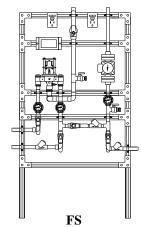
Megatron® with separate legs to floor to support the unit without hangers.
